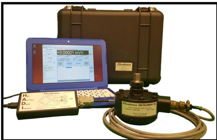
Direct reading in accordance to ASTM-E74 and ISO 376 when using a computer interface indicator and Morehouse custom software.
