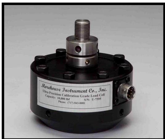
Morehouse load cells are available in several models. The Ultra-Precision model is the preferred choice for Calibration Laboratories. The susceptibility to eccentric loading is reduced by trimming the cell with the threaded adapter installed.
