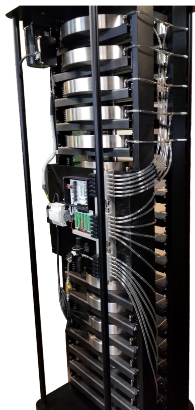
Figure 10: Pneumatic System Removes or Applies Weights
