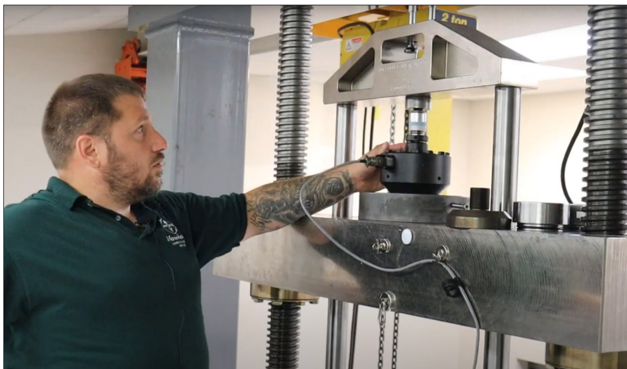
Calibration Technician Aligning a Load Cell with Adapters
