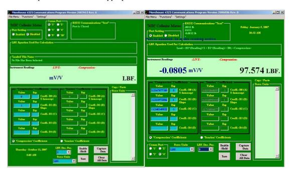
After the coefficients file has been loaded the screen should look like the one pictured left above. This example uses second degree inverse coefficients and is a universal load cell (both compression and tension) the calibration report issued will show what degree fit yields the lowest uncertainty.
