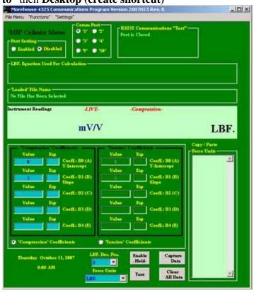
This is the screen that should now be seen. Before selecting Enabled the correct Comm Port should be selected and Coefficient files should be loaded from the File Menu. In this example the Comm Port will be set to '4' and an inverse coefficient file will be loaded.
