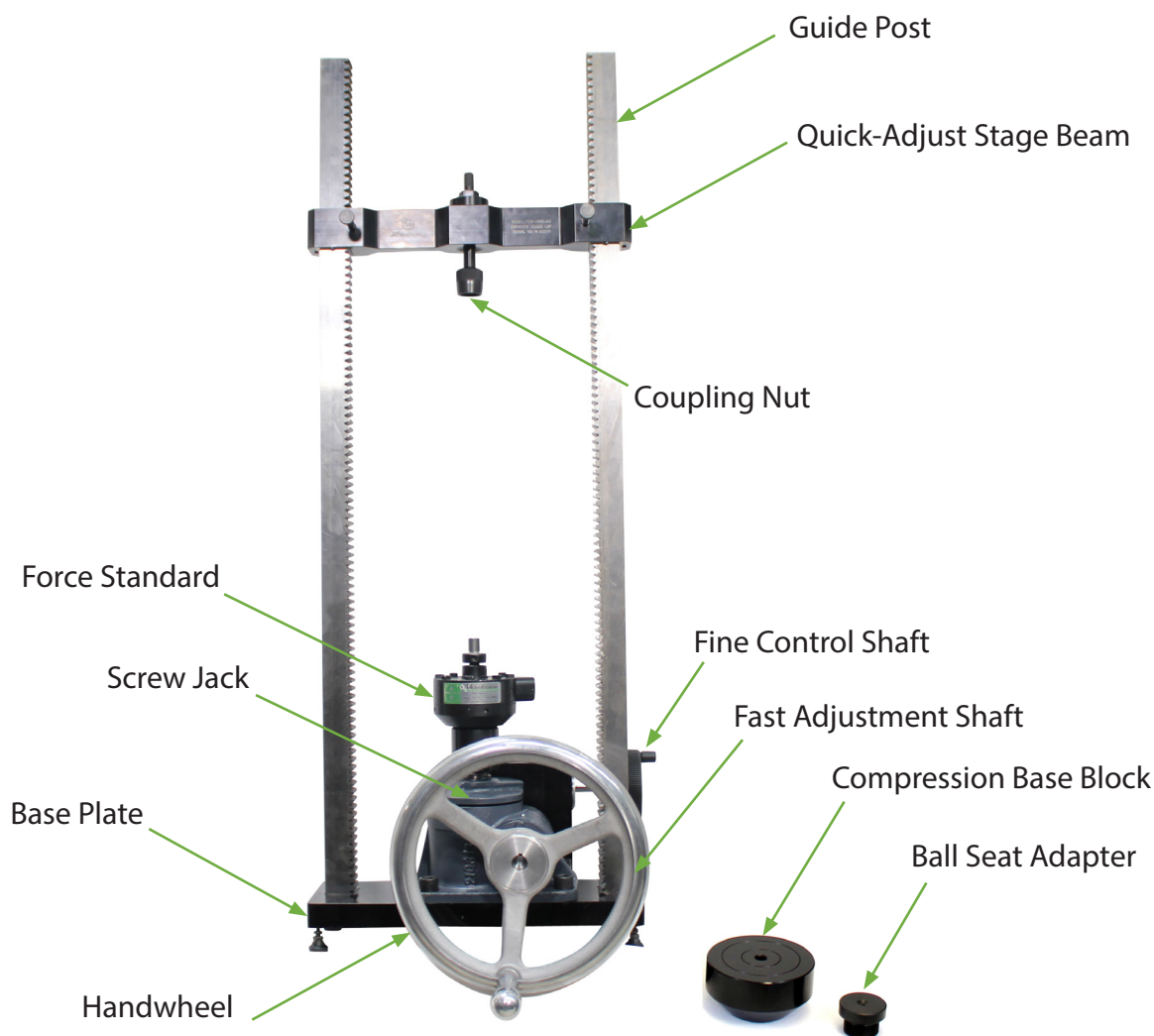
Figure 1: Standard Components of a Benchtop Calibrating Machine
