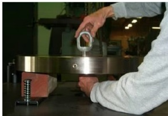
7/8"-14 Lift Eye Attached to Lift Rod #13
