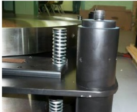
Hand Tighten Spacer & Loosen ¼ Turn
