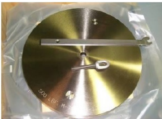
Tools Needed: Weight Lifter/Long Wrench, 7/8"-14 Lift Eye with 7/8"-14 Threaded Rod
