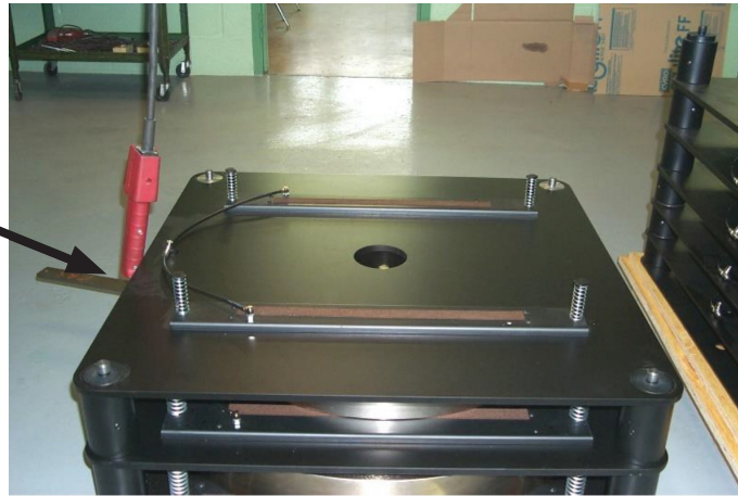
200 LB WT Lowered on to Lifter Pan
