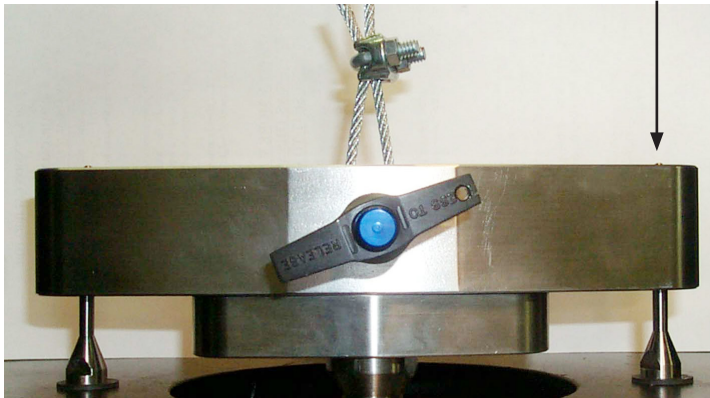
Highest Yoke Position...Top of Yoke Even with Top of Anti-Rotation Pins
