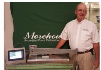
Picture of Bill Lane with Automated Torque System. Bill recently designed this system to eliminate ergonomic issues associated with manually lifting weights on a pan. The system is operated with a pneumatic cylinder and load cell. It is designed to be a retrofit to any current torque arm with weights.
